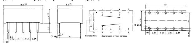
AL-D type (Double winding latching type)
