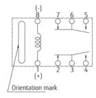
PC board mounting pad layout (TOP VIEW)
