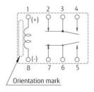
PC board mounting hole layout (BOTTOM VIEW)
