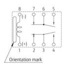
PC board mounting pad layout (TOP VIEW)
