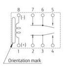
PC board mounting pad layout (TOP VIEW)
